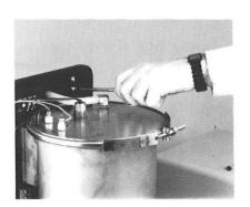
To service the electrical module: Unscrew with phillips screwdriver. Then unscrew four screws on back of furnace. Two are on top of the electrical module and two are
